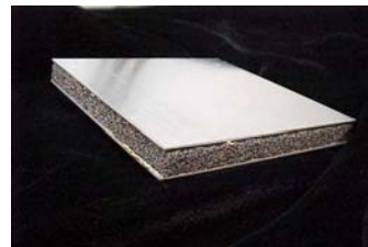
Al-face sheets joined to Gr-Foam with S-Bond.
