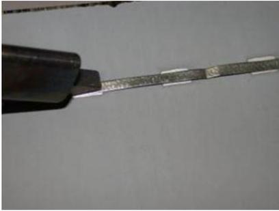
Figure 4. Thermasonic solder tip heating and bonding to Al-rear contact on PV cell.
