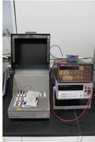
Figure 7. Multimeter test set up for measuring contact resistance and resistivity of soldered bus on PV cells.
